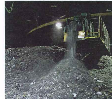
In a holding room, conveyors of ASR are dumped into piles, and then eventually weighed and loaded into the processing line.
