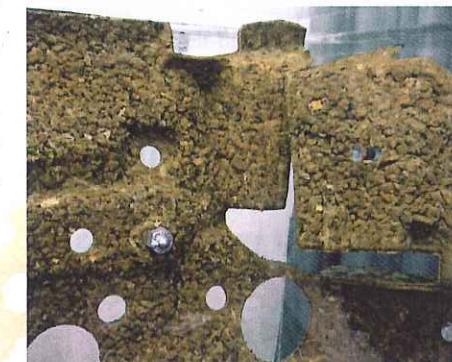
This frame is covered in flecks of orange foam that appear to have been sprayed upon the metal. It is in fact shredder residue which is turned into sound-proofing.
