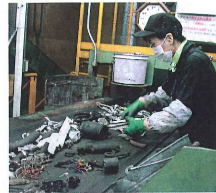
Hand-sorters are stationed just past a non-ferrous metals separator where they sift through fragments greater than 35 mm in size.
