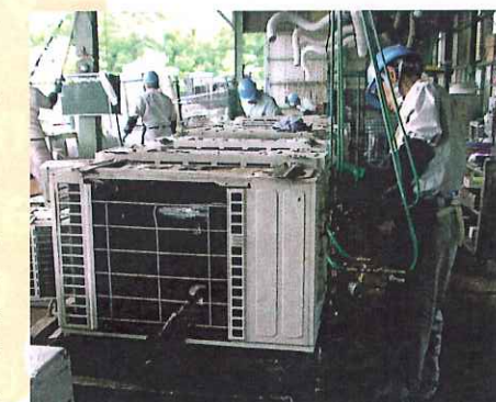
Workers are draining Freon from air-conditioners and refrigerators before the appliances are shredded.
