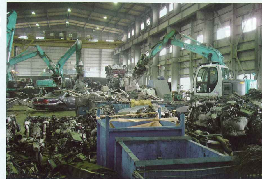
In one of Eco-R's scrap halls, hydraulic cranes rip and tear at the vehicle bodies and motors that couldn't be salvaged for re-use.
