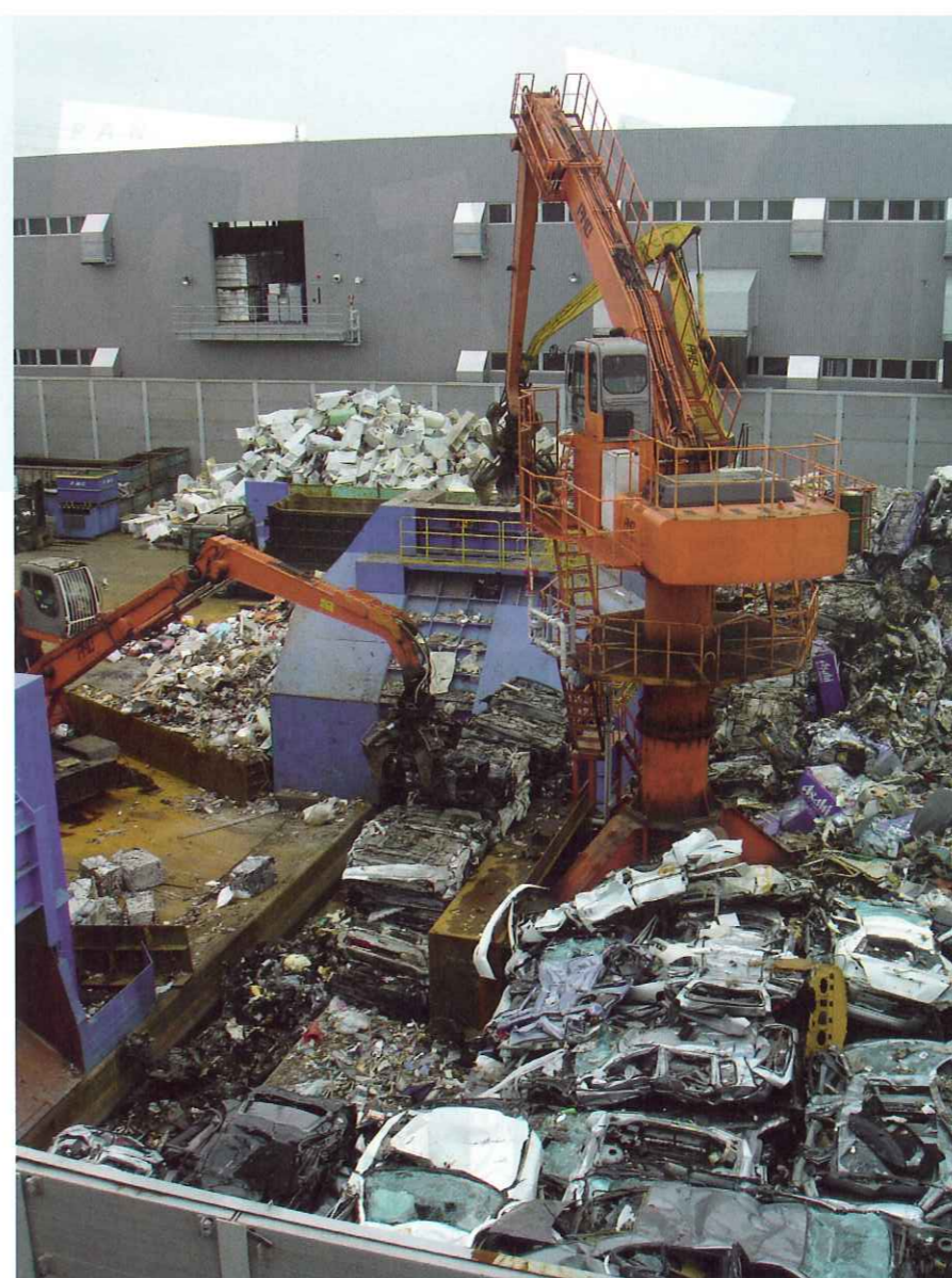
Flattened car bodies and stripped white goods piled loosely beside a pre-shredder at Phoenix Metal Group, East of Tokyo.
